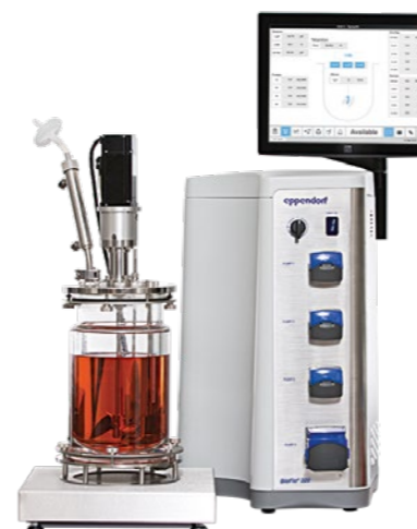
BioFlo® 320 0.6 – 10.5 L working volume (autoclavable), 0.25 – 40 L working volume (single-use)
