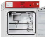
Interior and shelves made of stainless steel
