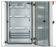
Inner door made of safety glass
