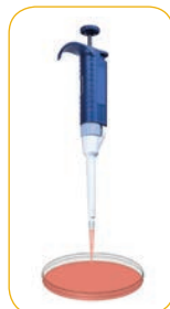
Aspirate sample into 1000µl tip
