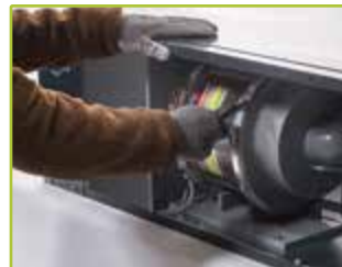
3 Insert the filter unit, fasten it and close the housing front
