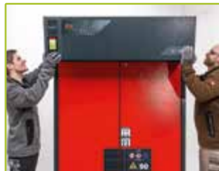
2 Place the recirculating air filter system on top of the cabinet and connect it to the cabinet ventilation
