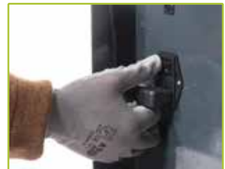
4 Plug in the low-temperature IEC power cable and switch on the device
