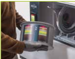
1 Unpack the device, open the housing front and remove the filter
